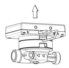
We always recommend detaching the calculator from the flow sensor.
