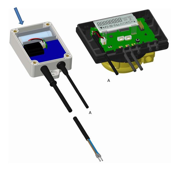
Only authorized technical personnel may connect the power pack to the 230 V mains supply and check it. When the meter detects external power supply the pictogram of a mains plug appears in the display lower left. Close the calculator.
