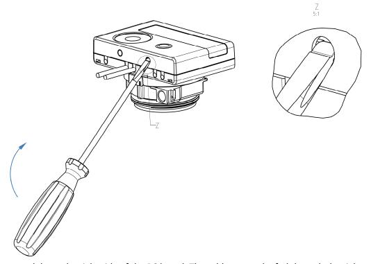
Plug the interface module on the right side of the PC board. The cables are to be fed through the rightmost cable feedthroughs into the calculator after removing the blind grommets. Close the calculator.
