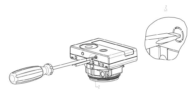
Then insert the screwdriver into one of the two openings at an angle of approx. 45° and carefully lift the handle up to approx. 90° (see picture 2). The upper housing piece of the calculator is then no longer latched on this side. Repeat this with the other opening. Now the upper housing piece can be taken off.
